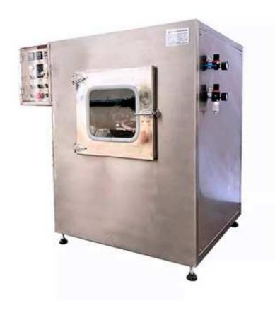
Fully enclosed tablet film coating machine has some advantages: such as easy operation; less dust; smooth and fine tablet surface; saving auxiliary materials and convenient maintenance. This machine is used for carrying out sugar coating and film coating to the core of Chinese and western medicine tablets. It integrates strong power, weak power, hydraulic pressure and pneumatic. It is the new type equipment that improved on the basis of the original sugar coating machine.
