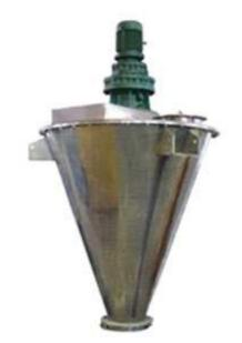
The Self-rotation of this machine is achieved by a set of motor and cycloid pinwheel reducer, non-Symmetry blending is achieved by two sets of screws as to let the large area mix and have fast mixing. It is especially used for mixing the materials with big difference of bulk density and mixing proportion.
