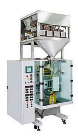
Automatic Filling Packing Machine - CC-1203 suitable for filling weighing and packaging various granular products, such as crude sugar, red beans, rice, green beans and feeding stuffs etc.
