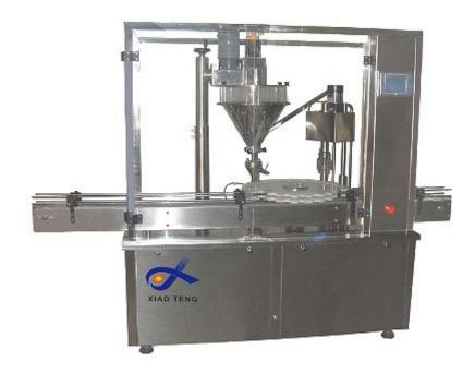
This all-in-one machine researched and developed on request of oversea customers integrates powder-filling and cap-putting functions. It can perform filling, cap-putting and cap-pressing (cap screwing) functions. It has compact structure and is easy to operate.
