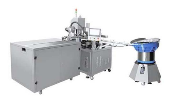
The powder pressing machine is applied to press the color cosmetic powder product, such as the powder cake, blush, eye shadow. In piece on the cylinder automatic powder, powder quantity can be adjusted in accordance with the powder compared to the corresponding
