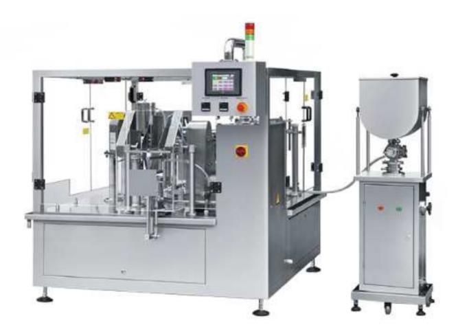
This line mainly installs rotary packing machine and liquid filling machine, suitable for packing all kinds of liquid, such as fruit juice, hand sanitizer, liquid detergent and so on.
