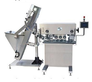
The capper PCL-15F is a reliable, high performance machine, designed in conformance with current and proposed GMPs. Having a small footprint, they are effective in maintaining the integrity of a clean room environment. Few change parts needed for different cap sizes (only the cap slide rail). The machine is designed for maximum efficiency and versatility. It utilizes the latest technology to automatically place and precisely torque a wide spectrum of cap types onto virtually any bottles type.
