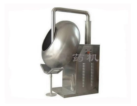
BY sugar coating machine is used for average coating and polishing of formed tablets and pills in pharmaceutical and food industries. It is also used for rolling and heating beans and edible nuts or seeds. In addition to this tablet coating machine, we also provide BYS series coating machine.
