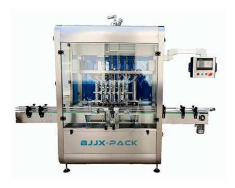
Liquid paste filling machine is suitable for filling various liquid, such as like shampoo, oil, laundry detergent, etc.
