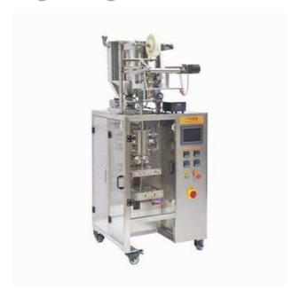
This stick machine can automatic measuring, making bag, filling, sealing, cutting off, batching number and output counting, suitable for viscous material such as honey, chocolate paste, etc.
