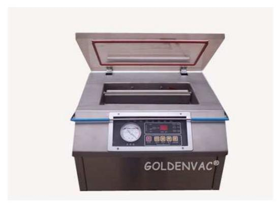
The vacuum packaging machine is designed for sealing contents in vacuum pouches Vacuum bags. It is equipped with an electronic pressure sensor to assure steady control of vacuum and gas packaging functions. Plus, a letter and number kit is included which will allow date and text message identification to be embedded in the seal of each package. A great way to set "freshness" markings.
