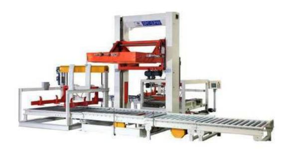
According to a certain order, palletize stacks the packed products (in box, bag, bucket) to the corresponding empty pallets through a series of mechanical actions so as to facilitate handling and transporting batches of products to improve production efficiency. Meanwhile it can use stack layer pad to improve the stability of each stack layer. Various forms designed to meet different palletizing requirements.
