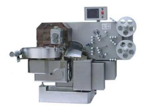
SWM300 Single Twist Packaging Machine is designed for high speed packing hard candy, milk candy, beef grain, preserved fruit into single twist style. Machine wrapping speed up to 350 per minute, depending on product. Machine of modern design, easy to clean and easy for maintenance. Fitted with double brush feed plate system, double paper feed reel holder for inner wrap or speedy change over of reels, air assisted paper feed system.
