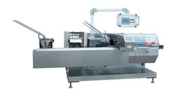
The Automatic Blister Cartoning Machine finished running by a series of photo-electro controller to make the machine stability and guarantee the packing quality. It includes leaflet automatic folding, canton opening and folding, products and leaflet feeding, batch number printing, sealing or hot-glue device. The machine can be linked with Tube Filling Machine, Blister Packing Machine, Shrink Machine, Three Dimensional Packaging Machine to form a complete production line.
