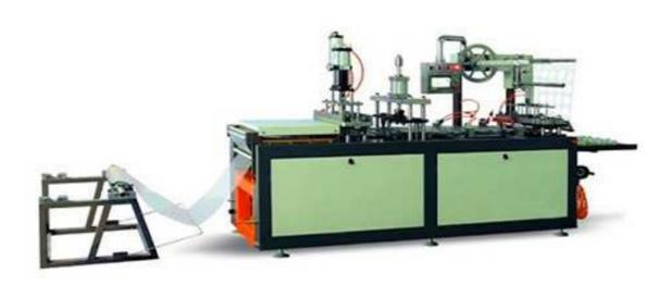
It is a small contact heat thermoforming machine which performing forming, hole-punch, cut&stack in 3 separate station. it is perfect for lid ,tray and clamshell with material of PET PS PVC PLA etc.
