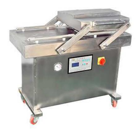
Ulike the single room vacuum packing machine, the DZ400/2S has double identical vacuum rooms that can be used interchangeably during operation. It's efficiency can reach 1.5-2times that of a single room, making it an ideal vacuuming equipment for small and medium-sized enterprises.
