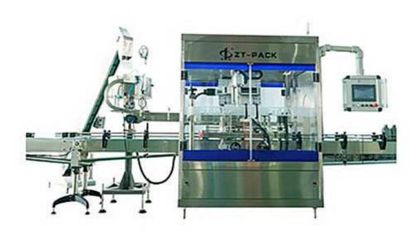
The fully automatic bottle capping machine is suitable for automatic capping of bottles with capacity ranges from 1L to 5L, it consist of lid unscramble, lid feeder, lid pressing system, as well as motion mechanism, conveying system and control system. Compared to ordinary capping machine that needs to be paused during the process for preventing the material from splashing out of the bottle, this bottle capping machine can implement the lid pressing process continuously and automatically.
