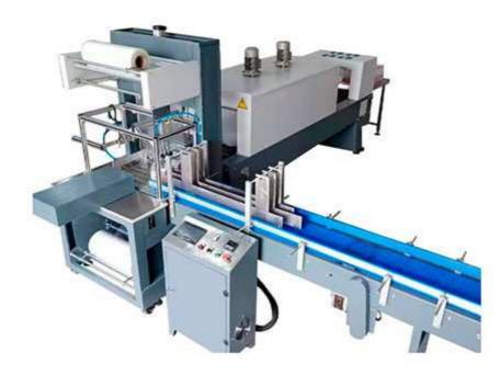
Specially designed for packaging production line of beer, beverage, pure water, fruit juice, dairy products, etc. With full automatic functions of bottle transfer and arrange, membrane packing, sealing and cut, shrinkage, cooling and shaping, etc.
