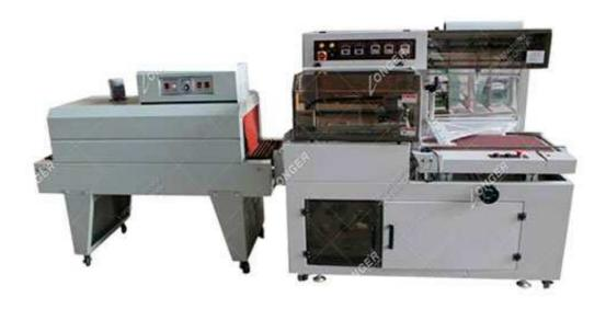
L sealer shrink wrap machine is specially designed for the packaging production line of beer, beverage, mineral water, juice and other semi-finished products. Heat tunnel shrink wrap machine can automatically complete the transfer and arrangement of bottles, film packaging, sealing, cutting, shrinkage, cooling and molding.
