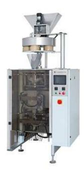
The machine is suitable for automatic packing particle materials like all kinds of sweets, chocolate, biscuits, peanuts, nuts, rice, millet, grain, seeds, pistachio, coffee beans, lima beans, sugar, salt and desiccant.
