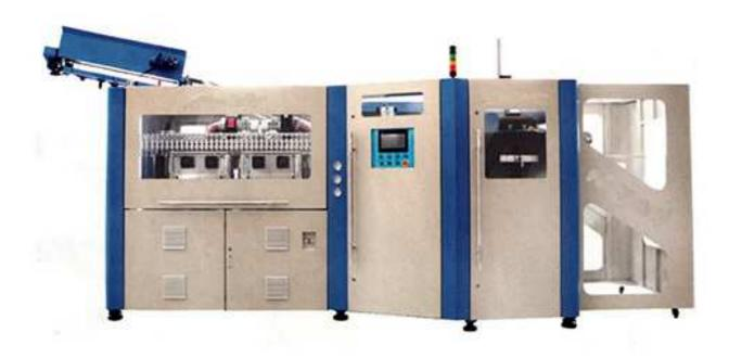
This drinking water Bottle Making Machine used for PET water bottle, hot-fill bottle, CSD drinking, oil and pesticide bottle.
