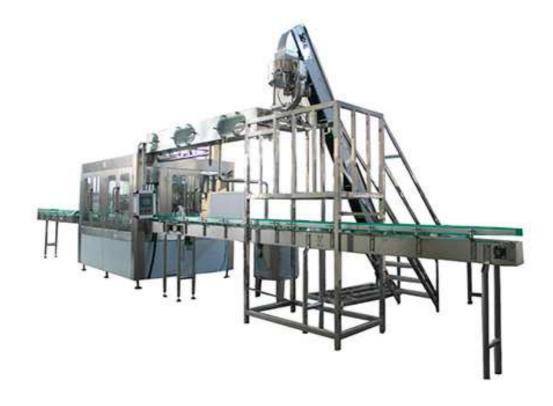
This XGF Wash-filling-capping 3-in-1unit: Beverage Machinery is used to produce polyester bottled mineral water, purified water, alcoholic beverage machinery and other non-gas beverage machinery. Beverage Machinery can finish all the process such as washing bottle, filling and sealing, it can reduce the materials and Outsiders touch time, improve the sanitary conditions, production capacity and economic efficiency.
