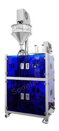
Chili powder packing machine can complete a series of processes such as bag taking, bag opening, blanking, sealing and coding.
