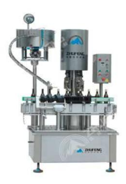
This automatic machine suit for sealing of disposable aliuminum wring type anti-theft caps. It can automatically arrange caps, drop caps, sleeve caps. Capping head use hard stainless steel, use four-wheel balance principle, uniform force, with high quality. Star wheel equip with automatic clutch, if bottle locked it can stop working automatically, bottle neck has automatic location equipment, stable performance, production speed fast, operation and maintenance convenient.
