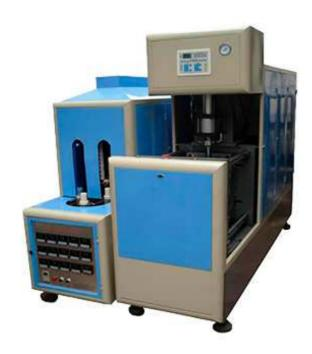
LINKS semi-automatic stretch bottle blowing machine with microcomputer controlling system. PET bottle blowing machine controls various technical parameter needed more accurately and more steadily. Only one person without special training operates PET bottle machine more easily and more safely.
