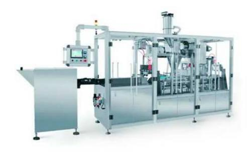
The coffee capsule filling machines are specifically designed for the needs of specialty coffee packing to provide more possibilities to ensure the freshness and shelf life of coffee capsules. The compact design of these coffee capsule filling machine allows for maximum space usage whilst saving labor cost.
