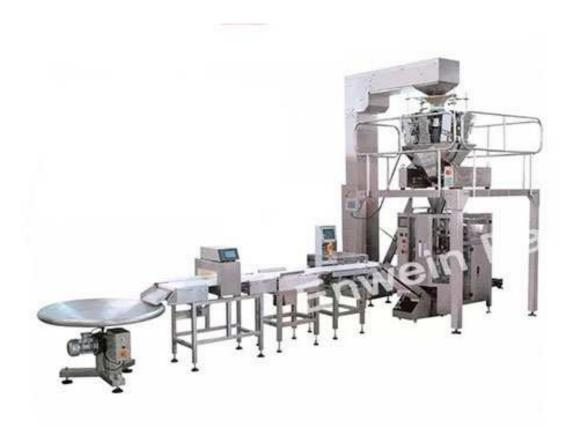
With a packaging speed of 15 to 35 bags per minute, the machine is suitable to package various freeze-dried fruit, such as dried strawberries, dried apple slices, banana chips, kins of nuts, etc.
