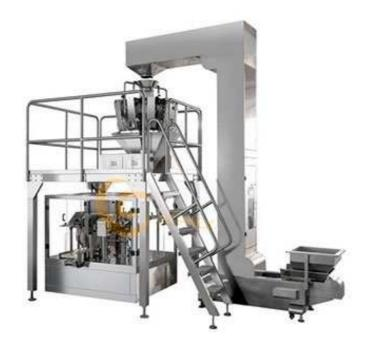
Grain Premade Rotary Packing Machine is a mini horizontal pre-made bag pick-up filling and sealing machine. It is an economical high speed bag packing machine that can finish 20pcs-40pcs packing per minute and also has the multi-function of zipper opening, European style punching and easy tear off. The packaging system consists of a mini multi-bag packaging machine, a multihead weigher, a Z-bucket elevator and a working flatbed.
