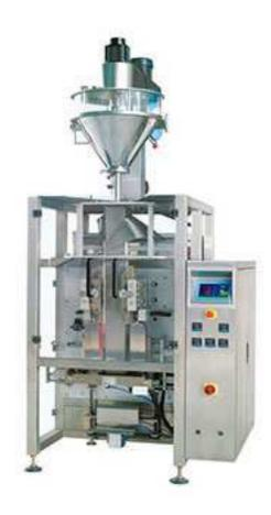
Suitable for pack food and chemical powder with stand up plastic bag, such as flour, milk powder, coffee powder, protein powder, starch, spice etc.
