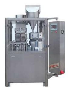
It adopts multi-bore dosing, batch-type rotating and speed frequency controlling. It includes whole capsule filling process: capsule sowing, separating, filling, un-separated capsule rejecting, closing, and filled capsule outputting. The machine is suitable for filling both powder and pellet.
