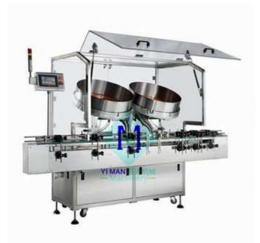
The Capsule/Tablet Counter Machine is widely used for accurately counting and filling of tablets, capsules and transparent products without change parts. It can be connected to other machines as an integral production line.
