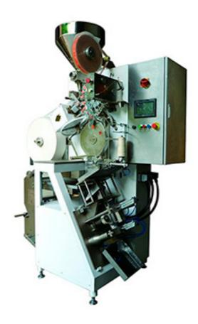
This automatic teabag packing machine can vary the quantity of teabags to be packed in an independent envelope. Our product can pack non-viscidity granule materials, CTC black tea, green broken tea, herbal mix granular formulations in various industry. It is controlled by PLC. Touch screen display. Operating easily.
