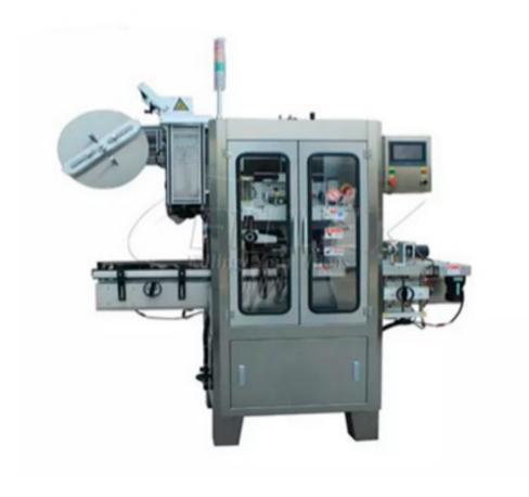
This machine uses a high speed machine equivalent PLC and positioning module and servo motor and inverter, touch screen automatic control, simple operation.
