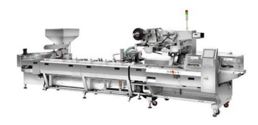
DXD-660Z High Speed Turntable Feeding Packing Line is used for high speed feeding and pillow type packing of bars products or products with regular shape and hard surface.
