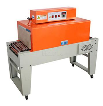
The far-infrared shrink packaging machine is the latest automatic continuous shrink packaging equipment in the domestic market. The shrink temperature and motor drive speed are stable and controllable, the adjustment range is wide, and there are instrument displays. The original roller auto-transmission device can work continuously.
