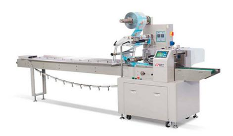
Flow wrapping or horizontal form fill seal (HFFS) is the process of making a horizontal bag from a single roll of film. Heat is applied to the bottom and ends of the film to form a sealed, flexible package already filled with products. Servo Packaging Machine for Food Products ZP-480S is suitable for a variety of products.
