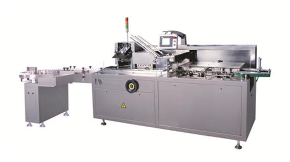
This carton packing machine can pack bottle which is round or flat, it also can pack eye drop bottle and so on.
