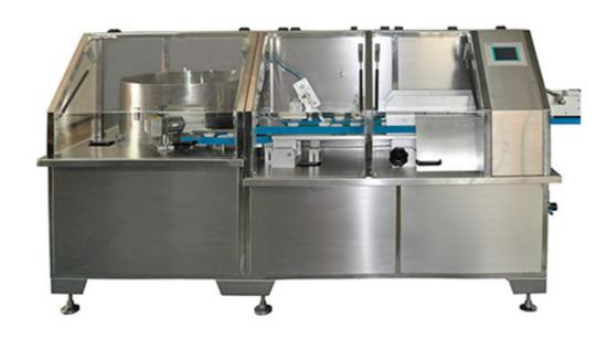
The machine is one member of our plastic bottle packing line. It can high speed supply to the bottle to next machine, such counting machine and filling machine, etc, suitability to other machine and is able to supply bottle to two producing lines simultaneously through two separate conveyors
