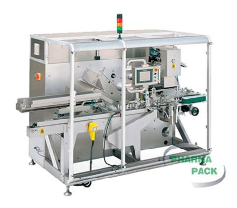
It can put the bottle, blister p board, material holder and other materials into the carton and then sealed box. If you use it with our folding machine, you can load the manual into the paper tray.
