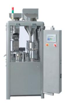
NJP-1200C Capsule Filling Machine can fill powder, granules and other materials into hollow capsules.
