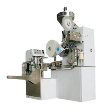
Tea bag packing machine Model DXDC8IV is our newest model, and features filling, heat sealing, threading, labeling and over-wrapping functions. Adopting sealing pads in place of the sealing rollers used in machines of previous generations, this new system greatly improves the machine's flexibility and enables use of different packaging materials. Main materials include paper/PE, plastic/foil/PE and plastic/PE.
