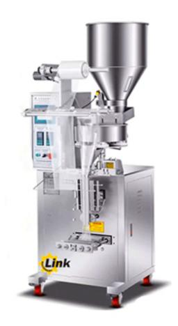
Automatic filling and sealing machine is suitable for various particles, such as grains, tea, spices, candies, biscuits, etc.
