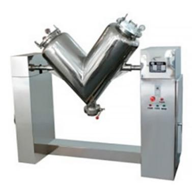
V type mixer or V shape mixer is mainly used for mixing dry powder material and granular substances in pharmaceutical, chemical, food, fodder, pottery, metallurgy and other industries. Raw materials can be input manually or through vacuum sucking. This high efficient mixer is made up of a container formed by two cylinders welded in an asymmetrical V shape.
