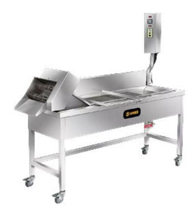
The AF-589 Series is equipped with a double-layered conveyor to deliver products in between, which enables them to be completely submerged in oil. Stirring or flipping is not needed. The Conveyor Fryer features digital temperature controller and thermal cutout to maintain stable temperature without compromising safety.
