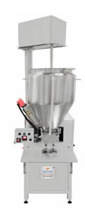
The Semi-Automatic Two Head Filling Machine consists of a main structure, product holder, hopper for filling material, piston, filling nozzle, foot-operated switch, electrical panel, motor & mains ON/OFF.
