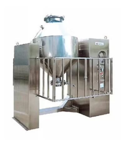
Double Cone Mixer is a lower cost mixing equipment for the powder, granule, lubricant adding, binder, seasoning's adding and mixing of western medicine, Chinese medicine and health food. Double Cone Mixer is uniquely designed to mix raw materials evenly, easy to operate and lower cost.
