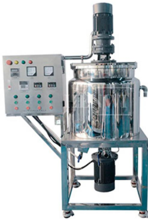
Homogenizing mixer machine has high-speed disperser, mixing and disperse viscously, solid and liquid, etc. various kind of raw material will be dissolved which is such as AES, AESA LSA, during liquid production which can save energy consumption and shorten production the and shorten production period. To produce liquid washing products, like shampoo, liquid soap, bath shower, dishwashing, hand washing, etc.
