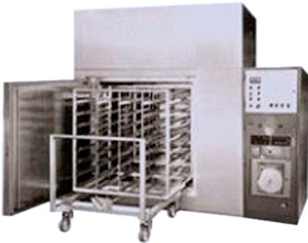
Vitro Pharma Machine provides Dry Heat Sterilizer which is used to sterilize items that might be damaged by moist heat or that are impenetrable to moist heat such as powders, petroleum products, sharp instruments.
