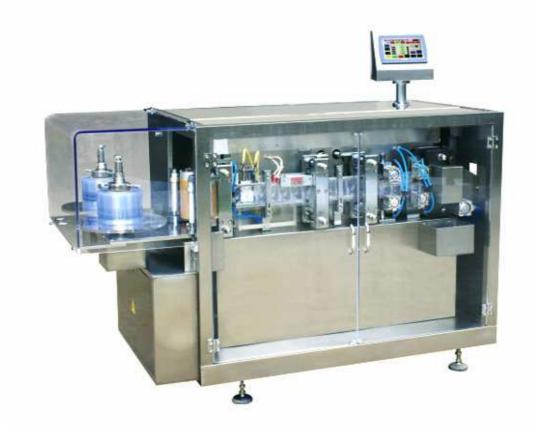
Take out the film; Plastic bottle-forming, filling, date printing, sealing and cutting can be completed automatically. Save cost and time.
