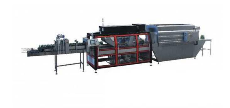
Shrink wrap machines apply heat to shrink a plastic film around a product. This process is often done by automated equipment, but manual and semi-automatic shrink wrap machines are also available. Shrink wrap machines cover the item, and then sent it through a heat tunnel or oven for shrinking.
